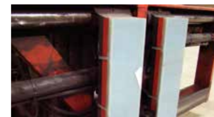
Soft backs with fastening slots
