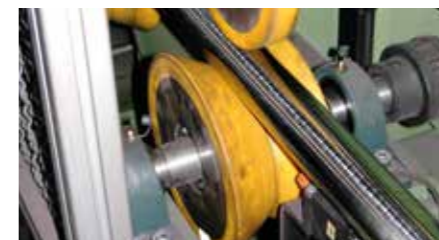
Guide and pressure rollers with replaceable inner core
