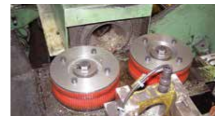
Heat-resistant and slotted draw-in rollers
