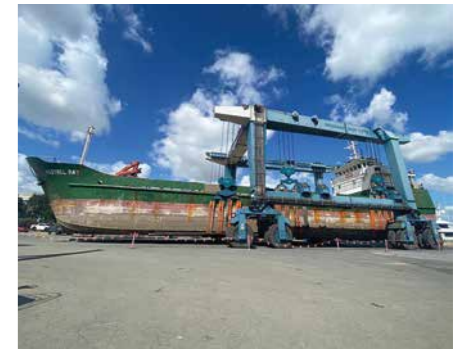
Application: Working ship with travel lift
