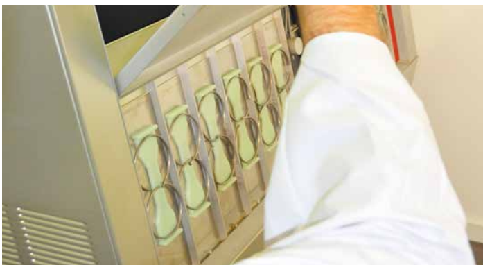
Weather tester for testing polymers in combination with light, temperature and humidity
