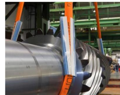
If the load moves laterally, a cutting movement takes place at the edge.
