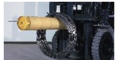
Pipe modules for forklift mandrels
