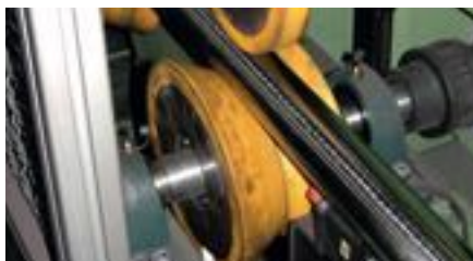
Guide and pressure rolls with exchangeable cores
