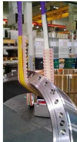
secuwave for protective sleeve for SpanSet PowerSTAR lifting sling as per sketch 1
