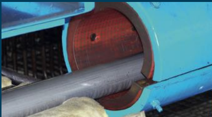
Lining for pipe raising systems
