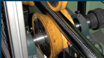
Guide and pressure rolls with exchangeable cores
