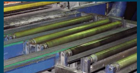
Rollers for the transport of sensitive profiles
